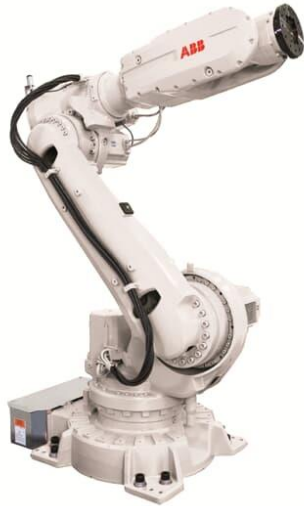
Fig. 1. Industrial manipulator ABB IRB 6620
