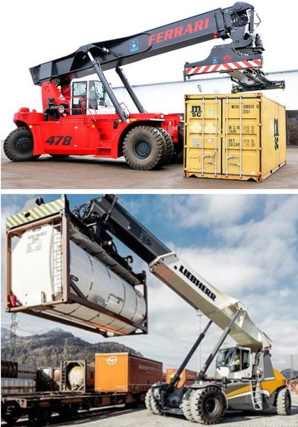
**Fig. 1.** Overload operations by reach stacker
