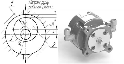
**Fig. 6.** Hydraulic oscillation generator: 1 – pulsator working chamber; 2 – spool; 3 – spool drive shaft
