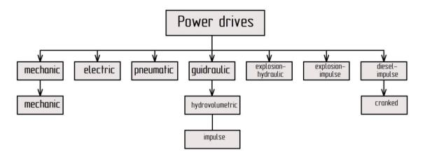
Fig. 2. Classification of power drives in construction machinery
