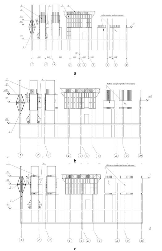
**Fig. 7**. Scheme of mechanized modules lifting during monolithic concreting: 1 – pilon; 2 – mechanized module; 3 – reinforcement; 4 - moving platform; 5 - panel (static) formwork; 6 - static platform
