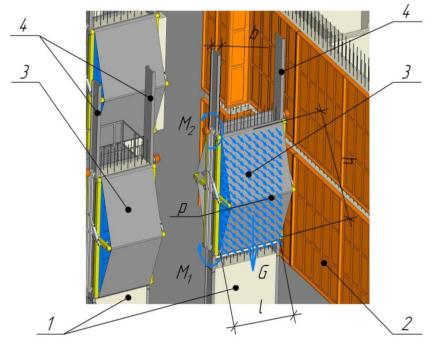
Fig. 1. Example of determination of forces for mobile formwork:
