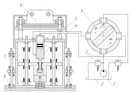
Fig. 5. Non-Battery dynamic hydraulic drive with a crane-type spreader:
