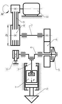
**Fig. 3.** Crank drive: 1- output drive link; 2- working body; 3- connecting rod; 4- crankshaft; 5- coupling; 6- gear transmission; 7- shaft; 8- flywheel; 9- V-belt transmission; 10- engine; 11- brake
