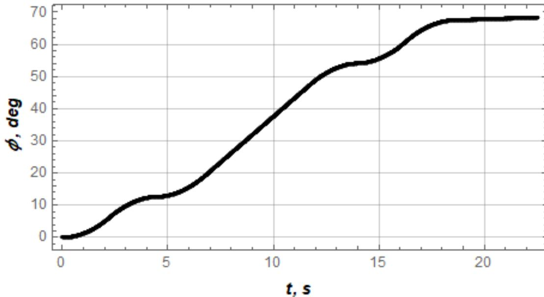
**Fig. 4.** Graphical representation of the boom position throughout the motion of the boom system (for the first experimental scenario)
