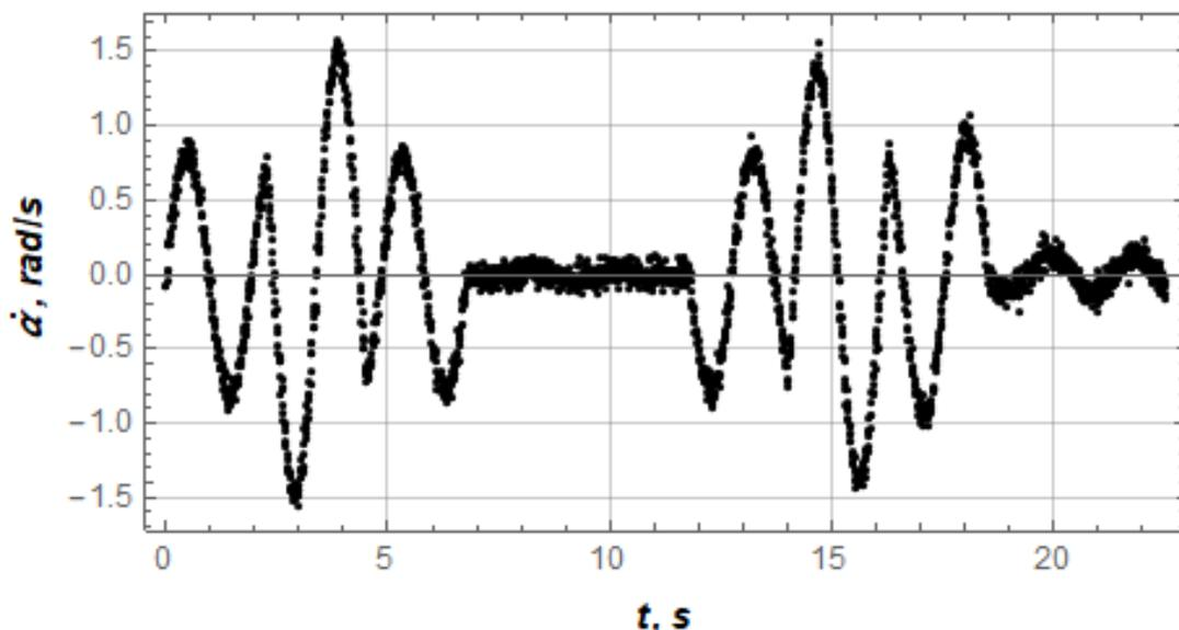
**Fig. 3.** Graphical representation of the angular speed of load deviation from the vertical over the entire motion range of the boom system (for the first experiment variant)
