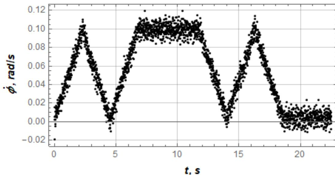
**Fig. 5.** Graphical representation of the boom angular velocity throughout the motion of the boom system (for the first experimental scenario)
