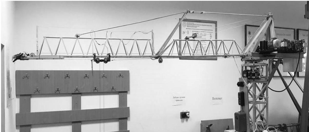
**Fig. 1.** Experimental laboratory setup of the tower crane
