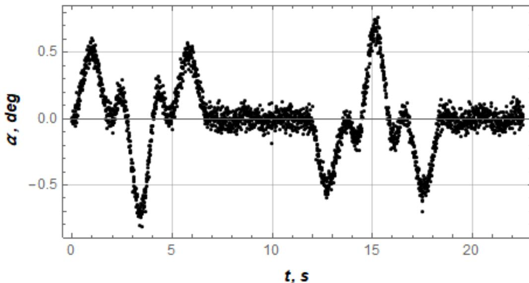
**Fig. 2.** Graphical representation of the load deviation angle relative to the boom over the entire motion range of the boom system (for the first experiment variant)
